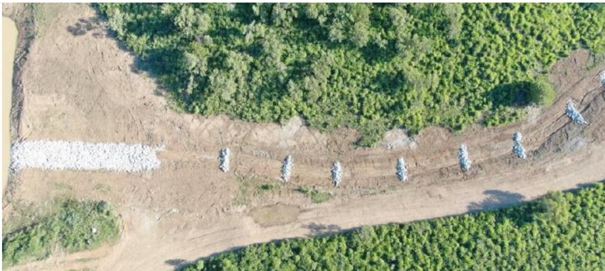
Figure 7 SB23A inlet was rock lined, and the drain had rock check points installed to avoid erosion in the drain
