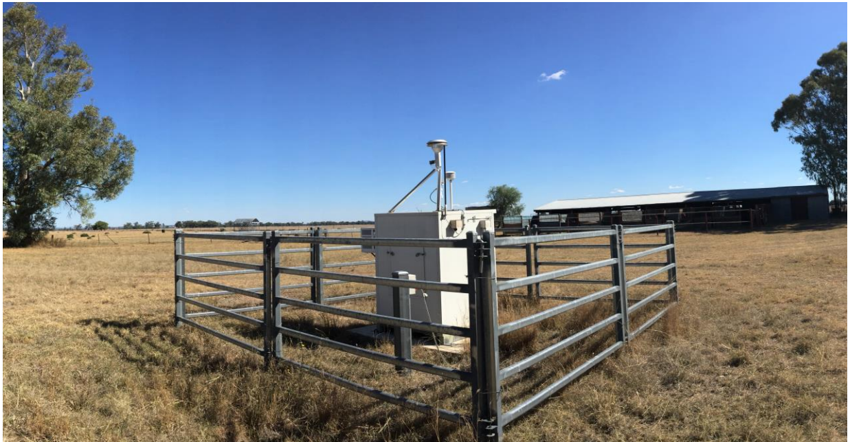
Figure 1: TEOM installed at Flixton property
