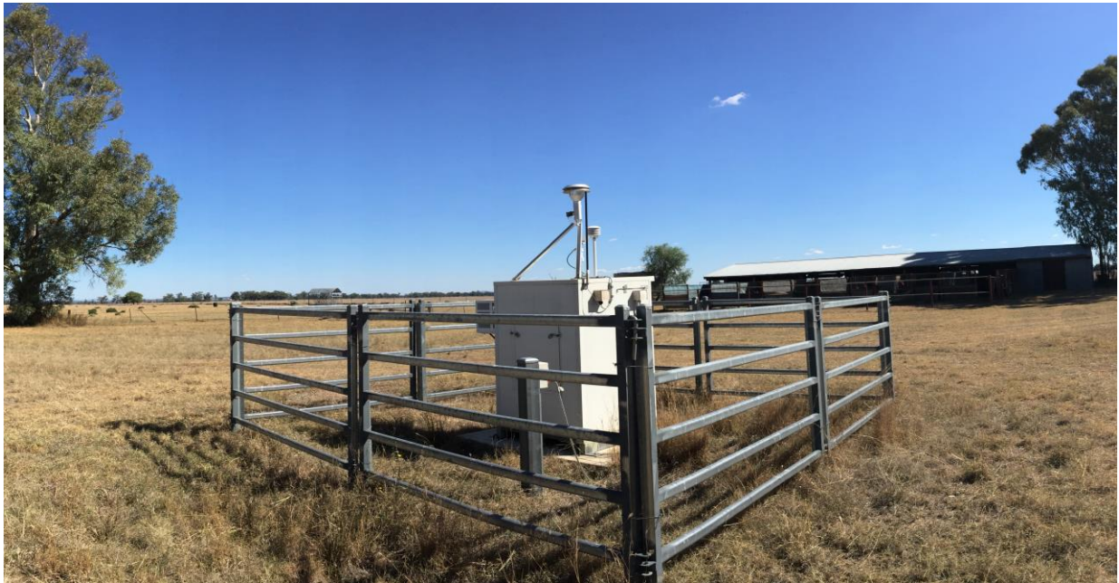
Figure 1: TEOM installed at Flixton property
